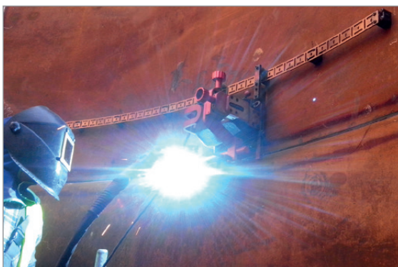
Guide flexible 185 cm (6ft) 1 pc Rayon minimum de courbure: 1.0 m (3.3 ft) PRW-0466-50-01-01-0
